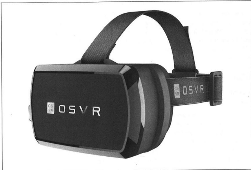
Figure 2-5. Razer's headset, based on the OSVR open specification
