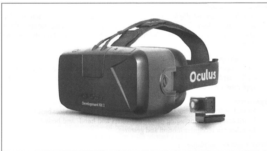
Figure 1-2. The Oculus Rift head-mounted display, Development Kit 2
