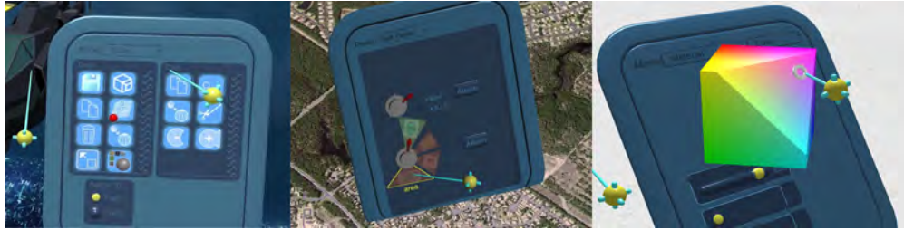
Figure 28.8 Three examples of hand-held panels with various widgets. The left panel contains standard icons and radio buttons. The center panel contains buttons, a dial, and a rotary menu that can be used as both a ring menu and a pie menu. The right image contains a color cube that the user is selecting a color from. (Courtesy of Sixense and Digital ArtForms)
