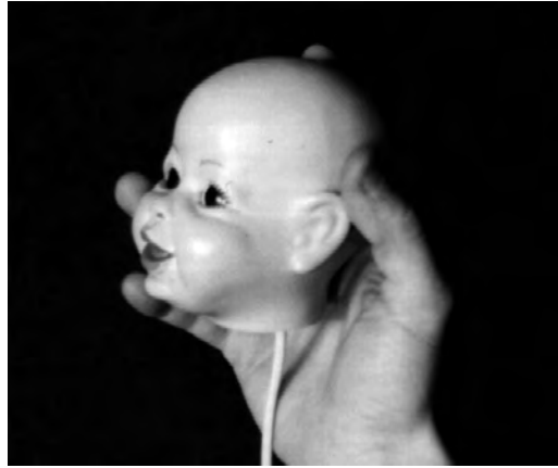
Figure 28.4 A physical proxy prop used to control the orientation of a neurological dataset. (From Hinckley et al. [1994] )
