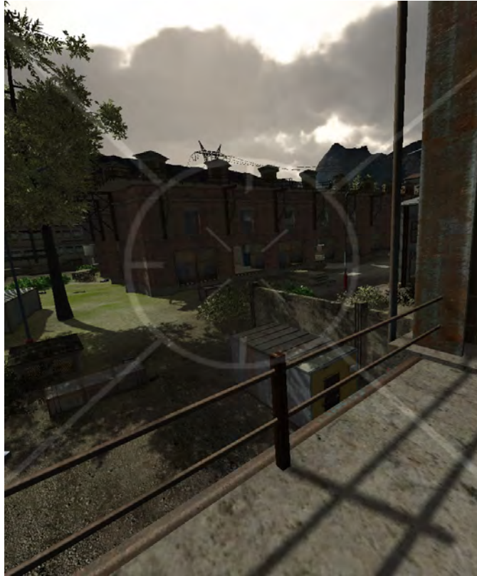
Figure 26.4 A heads-up display in the head reference frame. No matter where the user looks with the head, the cues are always visible. (Courtesy of NextGen Interactions)
