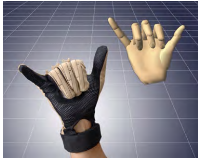
Figure 27.4 The CyberGlove is an example of a hand-worn device. (Courtesy of CyberGlove Systems LLC)
