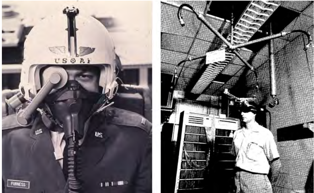
Figure 2.11 The Wright-Patterson Air Force Base head-mounted display from 1967 (courtesy of Tom Furness) and the Sword of Damocles [ Sutherland 1968 ]
