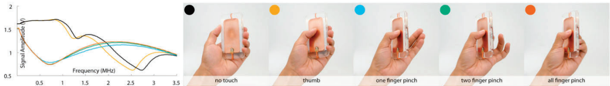
Figure 8: Capacitive profiles for enhancing touchscreen interaction with a hand posture sensing.
