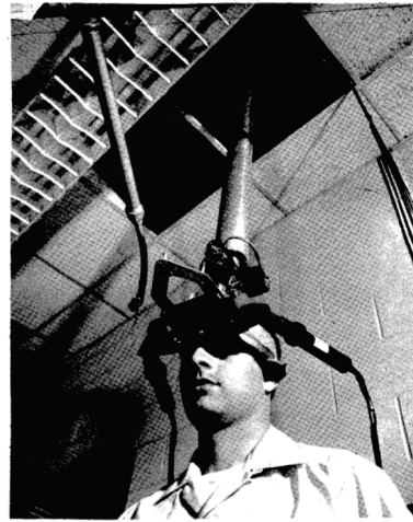
FIGURE 4—The ultrasonic head position sensor in use
