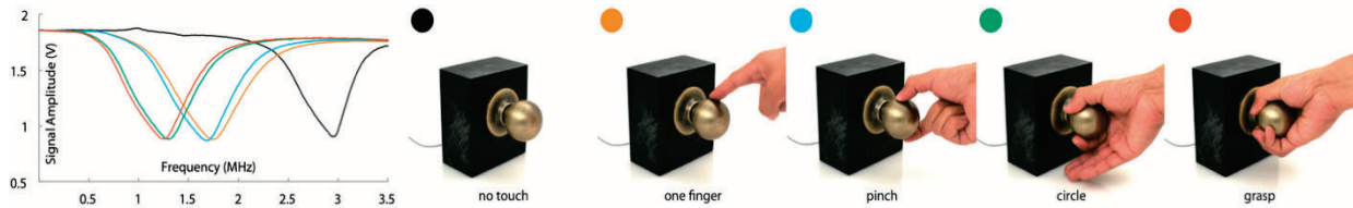
Figure 6: Capacitive profiles for making objects touch and grasp sensitive (doorknob example).
