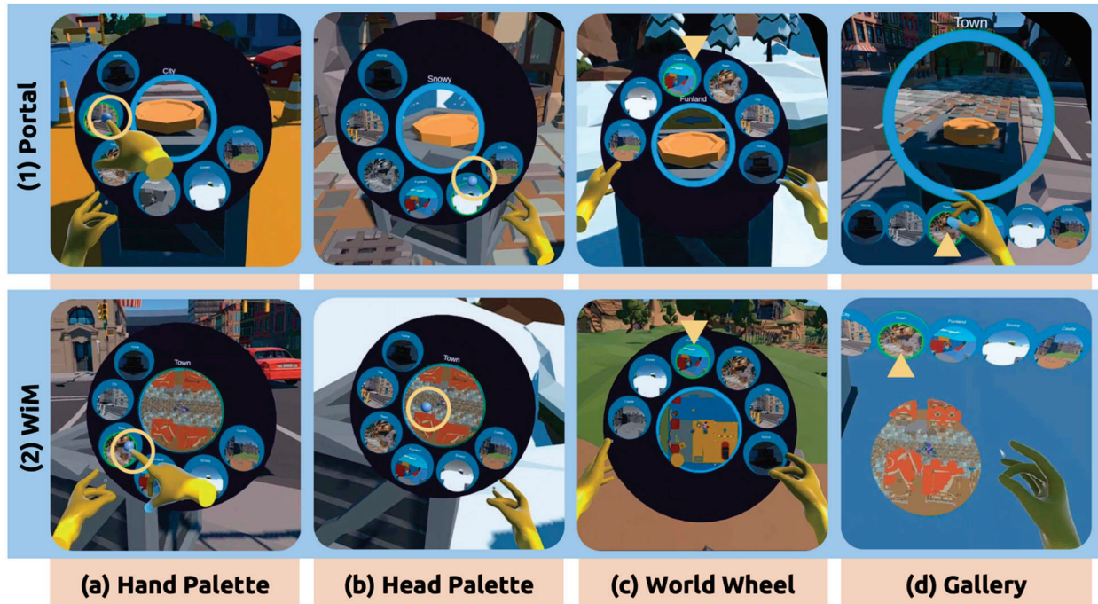
Figure 2: Eight virtual world switching interfaces evaluated in our study. Two preview patterns are used: (1) Portal and (2) World-in-Miniature (WiM). Four interaction techniques were derived: (a) Gallery, (b) Head Palette, (c) Hand Palette, and (d) World Wheel. The selected environment is indicated by a yellow arrow—(a) and (d)—or a blue spherical cursor—(b) and (c). The latter is highlighted with a yellow circle for clarity.
