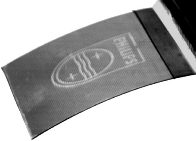
Figure 18.12 Photograph of an addressed paintable LCD. The Philips logo was activated by direct addressing of the in-plane switching electrodes. The total thickness of this paintable LCD with two TCF sheets is about 430 \mu\text{m}
