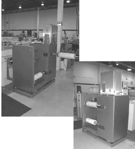
Figure 21.6 Web handling: Northfield Automation's unwind/rewind for develop, etch, strip (DES)
