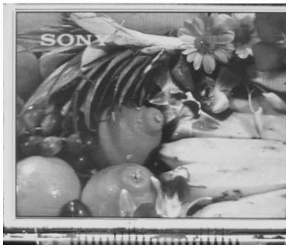
Figure 23.14 An image displayed on the plastic transmissive color LTPS TFT LCD. This 1.5 in. diagonal panel weighs only 0.5 g
