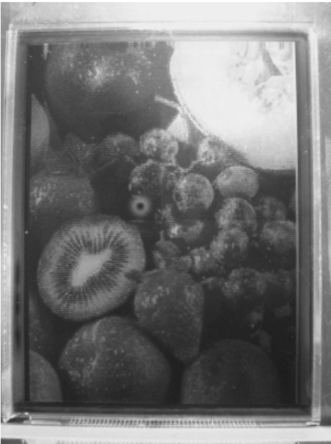
Figure 23.15 An image displayed on the 3.8 in. plastic reflective color LTPS TFT LCD. This panel weighs only 3 g
