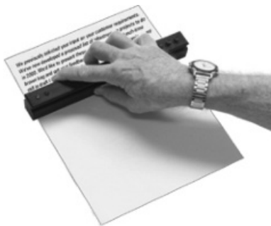
Figure 20.14 Handheld stylus wand printer, depositing image-wise charge on the islanded plastic surface of an electronic paper sheet
