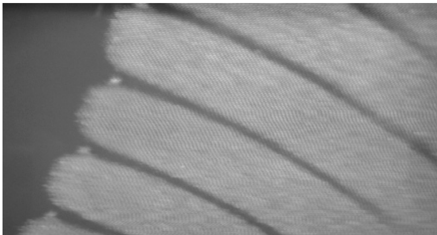
Figure 20.16 Flash-illuminated video image of a spinning disk showing the Taylor instability. The Taylor instability generates jets that become bichromal beads in the Gyricon bead generation equipment
