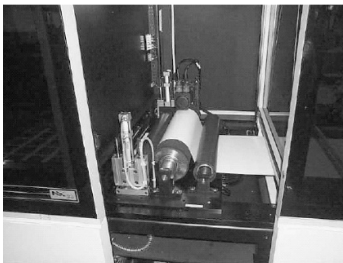
Figure 21.10 A web advance mechanism integrated into an Olec expoler
