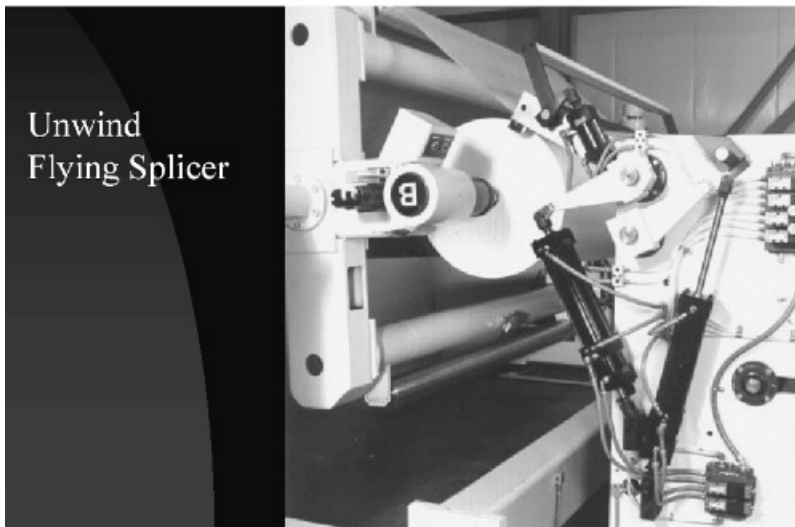
Figure 21.16 Decreasing waste and increasing productivity: web accumulator for “zero-speed” splicing
