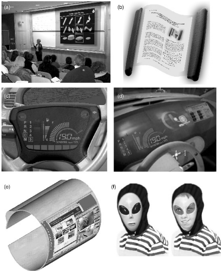
Figure 1.3 Various flexible flat panel display concepts: (a) a direct-view large-area screen; (b) a rollaway display system; (c) an odd-shaped display integrated in a steering wheel of an automobile; (d) a permanently conformed display covering the entire dashboard of an automobile; (e) a permanently conformed display that securely fits around the wrist; and (f) a child's switchable mask. Renditions courtesy of Suraj Gorkhali, Brown University
