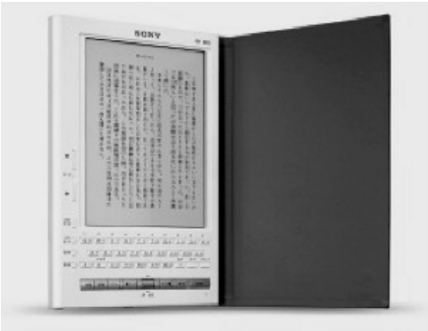
Figure 19.9 Sony Corporation’s LIBRIe electronic reader with E Ink’s microencapsulated electrophoretic imaging film in a display module made by Royal Philips Electronics
