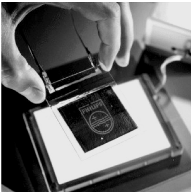
Figure 18.8 A photograph of an LCD produced by the PES process. The paintable LCD has been provided with a coatable polarizer. It was operated in the transmissive mode (normally black) by using a backlight/polarizer combination. The Philips logo was activated by direct addressing
