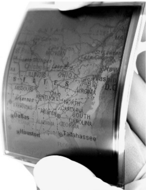
Figure 23.16 Displayed image on curved reflective color TFT LCD. The radius of curvature is about 75 mm
