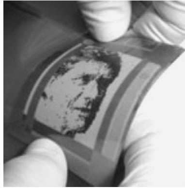
Figure 19.18 All-plastic display made using a microencapsulated electrophoretic imaging film from E Ink and an active-matrix backplane made by Plastic Logic. Courtesy of Plastic Logic Limited
