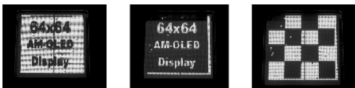
Plate 15.3 Active matrix OLED display on plastic: monochrome, 150 °C, a-Si TFT on heat-stabilized Teonex Q65 PEN, 64 × 64, 80 dpi
