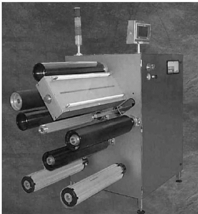
Figure 21.8 Web handling: Northfield Automation offers options such as dual material shafts, dual interleaf, and accumulation
