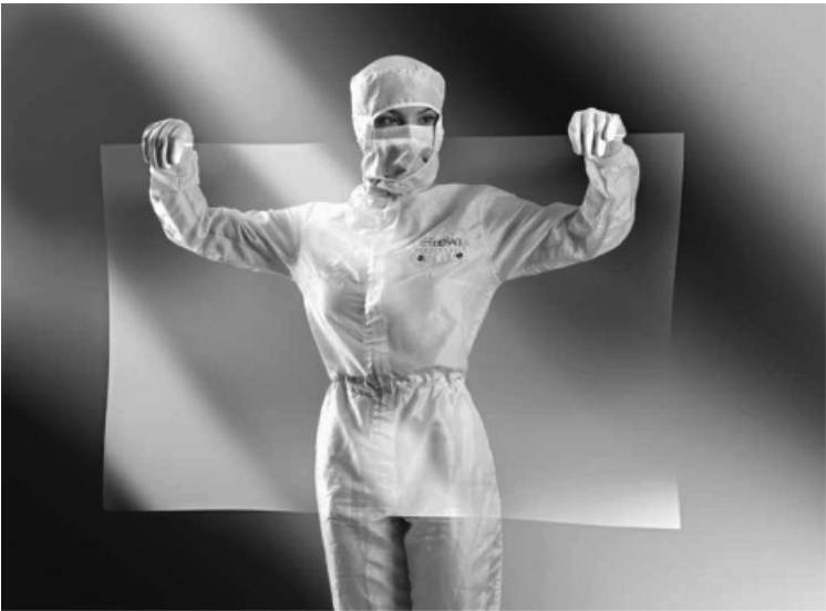
Figure 3.6 Large thin glass sheet, 50 \mu\text{m} thick, produced by the DD technology
