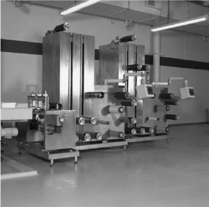
Figure 21.12 Dual rewind with inline slitting (28 in web to two 12 in webs)
