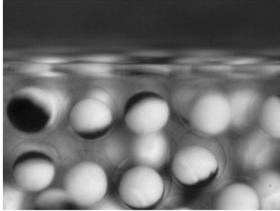
Figure 20.2 A photomicrograph of the edge of a Gyricon sheet having the same aspect as Figure 20.1
