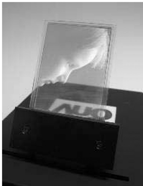
17.14 Transparent 2.4 inch QVGA display from AU Optronics Corporation using an IGZO backplane. The transmissivity is 45%. 15
