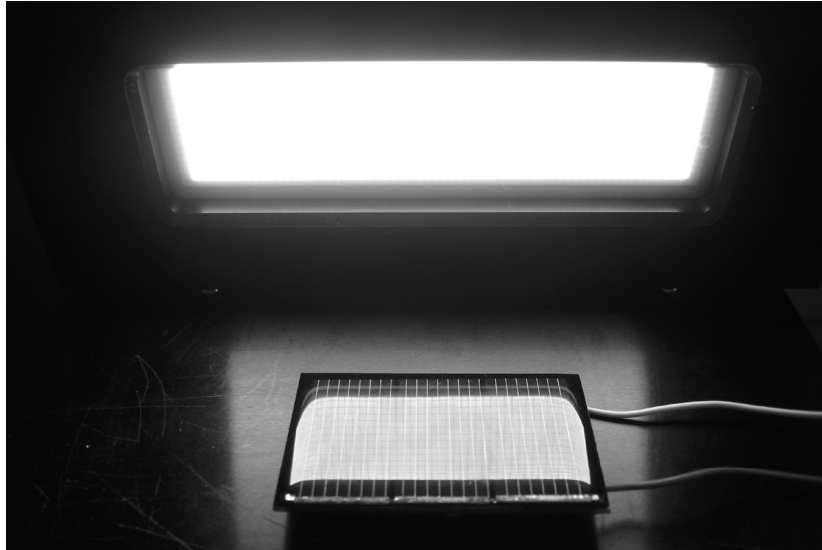
19.12 The test setup; the OLED panel sheds white light on the reference solar cell. (Source: Reprinted, with permission, from Park et al. (2010). Copyright © 2010 Institute of Electrical and Electronics Engineers.)
