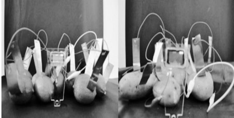
14.10 Lemons and potatoes are able to drive OLEDs.
