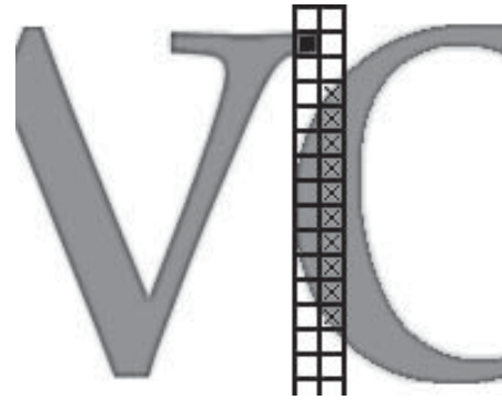
Figure 4: Distinguishing two characters from each other. The all-black square is a pixel that belongs to the connected component that comprises the current character. Since none of the pixels belonging to the next character touches the current character, an ending location is set here.
