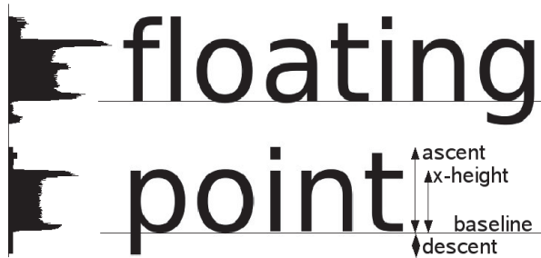
Figure 3: Two lines of text and their projections (on the left). Also illustrated are the length measures x-height, ascent and descent. In the proposed OCR system, these parameters are found by traversing the projection from top to bottom.
