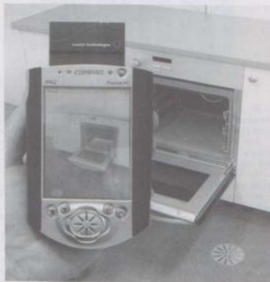
Figure 12: Prototype of the AR-PDA: The real image of an oven is augmented with a virtual telescope trolley
