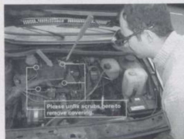
Figure 2: Assembly instructions are inserted into the users field of view via a head mounted display
