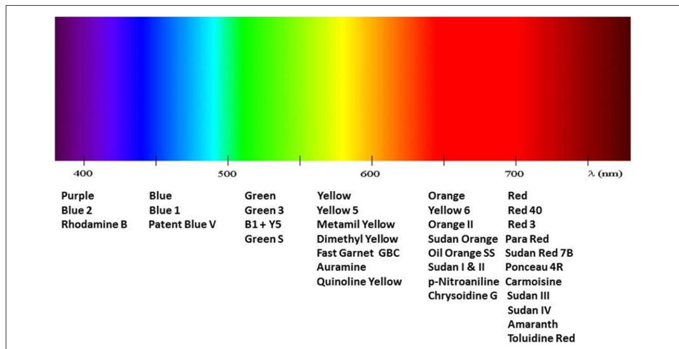
Figure 8–Potential adulterants to colorants from natural sources or food coloring materials based on their visible spectrum and color characteristics.
