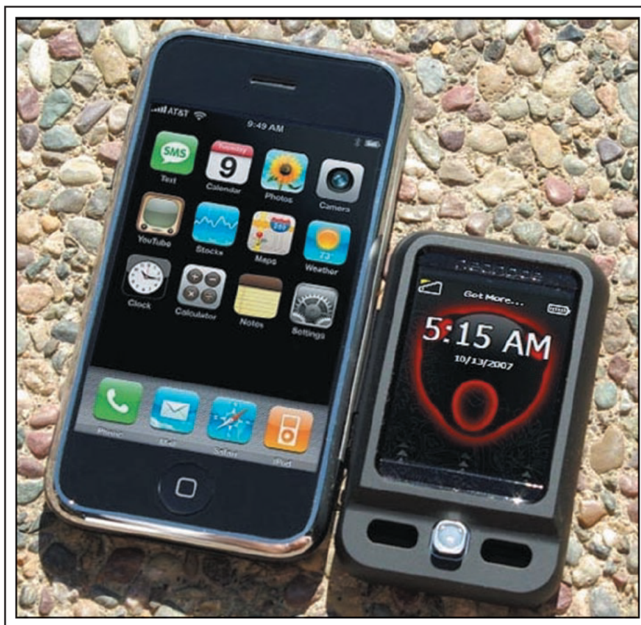
Fig. 2: The Apple iPhone with projected-capacitive touch (left) and the Neonode N2 cell phone with conventional optical touch (right). Photo courtesy of PenComputing.com.
