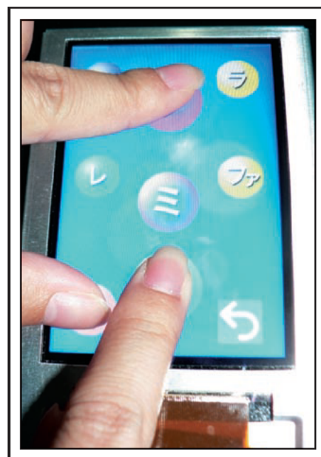
Fig. 5: Sharp's 3.5-in. LCD with in-cell light-sensing optical touch. Photo courtesy of Nikkei Business Publications Tech-On!
