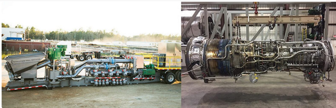
Right: A fully assembled pressure-pumping unit on its tractor-trailer. Left: A natural gas-burning turbine developed by General Electric, a variation of an aircraft engine, just prior to delivery and installation. Source: Evolution Well Services.
