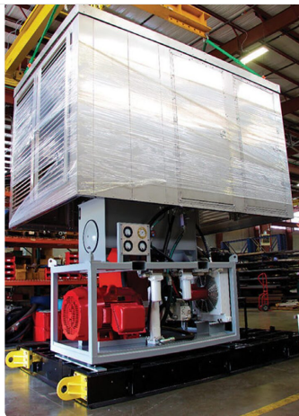
This self-contained power system being assembled outside of Houston was designed to replace more than a dozen pieces of equipment from the fracturing job site by supplying compressed air, electricity, and hydraulics. Source: MGB Oilfield Solutions.
