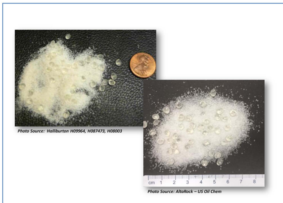
Figure 3—Example of bimodal PLA diverting agents
