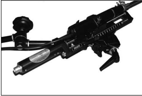
Fig. 13. Type 1850 and Pullback Mover UA0552 mounted on Variable Friction Arm UA0553
