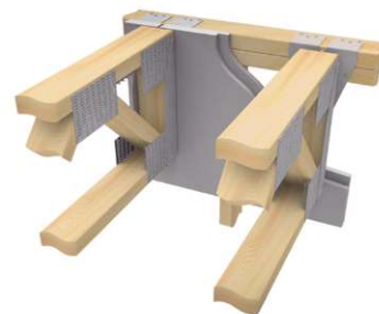
Typical FWH stud wall with (2) layers of 5/8" gypsum wallboard installation
