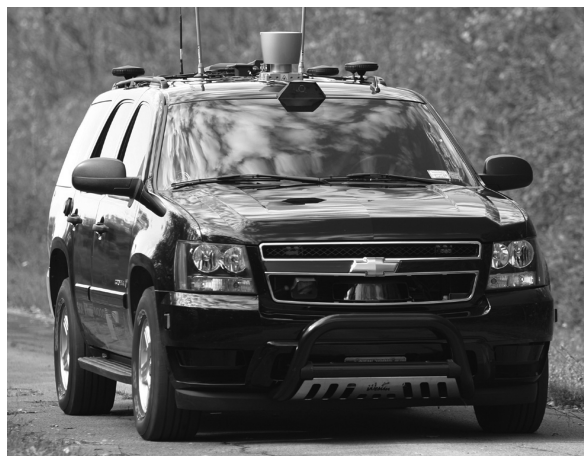
Fig. 1. Cornell University's Skynet, an autonomous Chevrolet Tahoe that completed the 2007 DARPA Urban Challenge. Skynet uses a tightly-coupled GPS/INS pose estimator implemented as an ESRIF.
