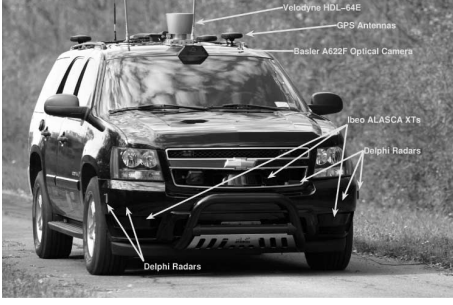
Fig. 3. Proposed tracking algorithm is implemented in real time on Cornell University's "Skynet," which is an autonomous 2007 Chevrolet Tahoe that completed the 2007 DUC.
