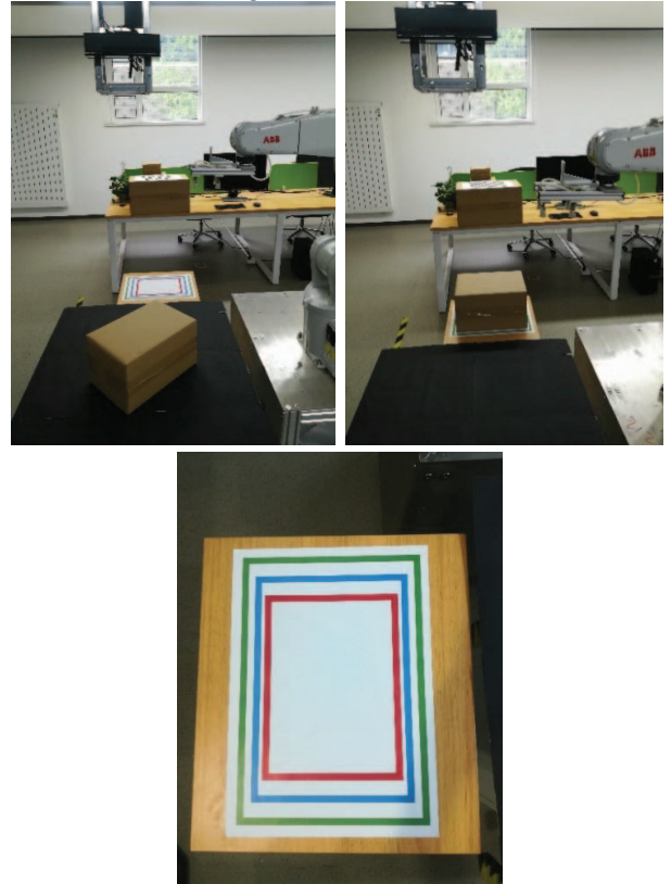
Fig. 6 Pick and place experiment. (Top-left) The box's state before picking. (Top-right) The box's state after before picking. (Bottom) Limited error for picking and placing to boxes with different size. If the box is placed inside the corresponding rectangle, we consider the picking up and placing down is successful.
