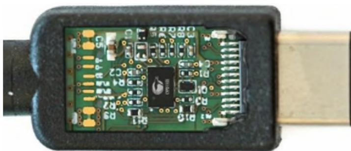
Figure 11. Type-C EMCA Plug with CCG1
