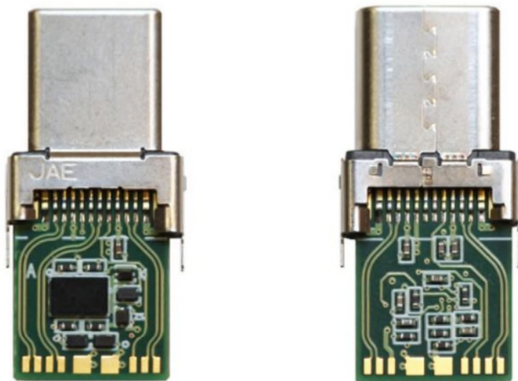
Figure 29. Complete CCG1-Based Cable Paddle Board Reference Design
