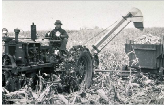
Figure 10. Corn harvest with a tractor-drawn corn picker.
