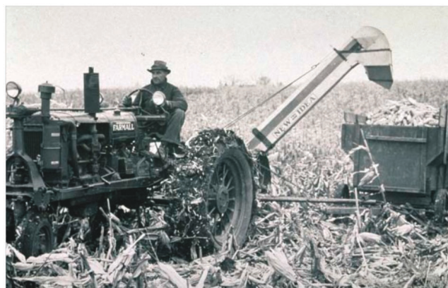
Figure 10. Corn harvest with a tractor-drawn corn picker.
