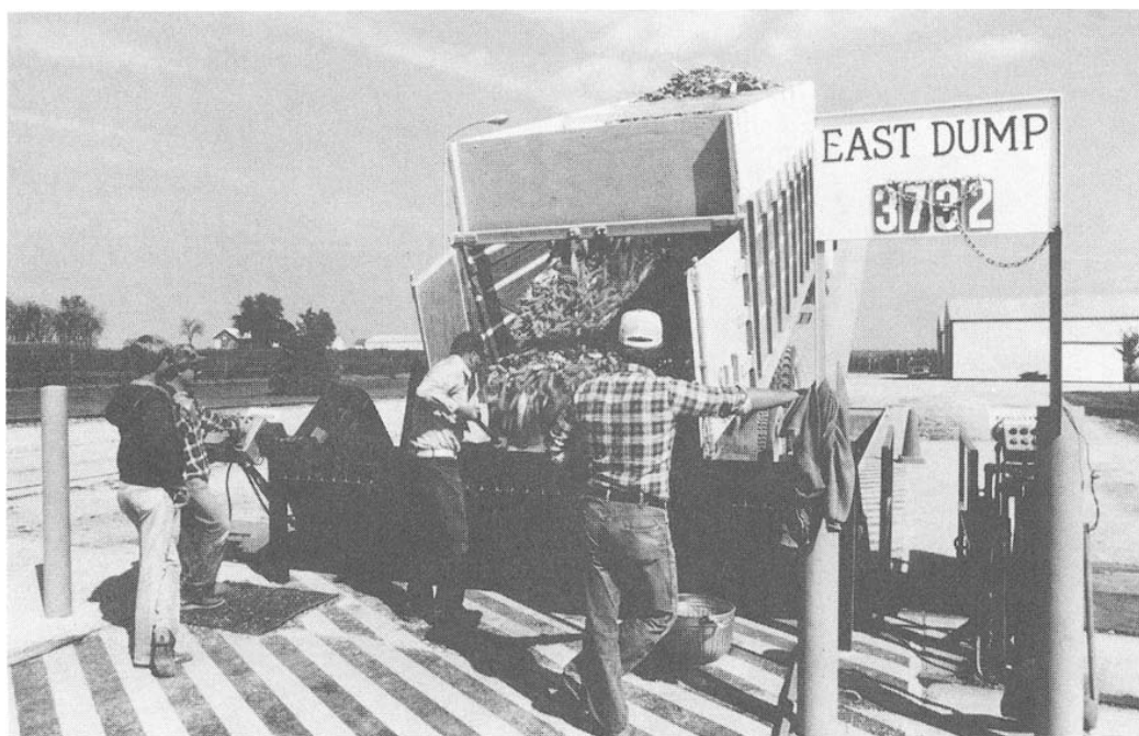
Fig. 9-8. Unloading seed corn at the green corn receiving area at a production plant. The ear corn is conveyed from this area to the husking and sorting building.
