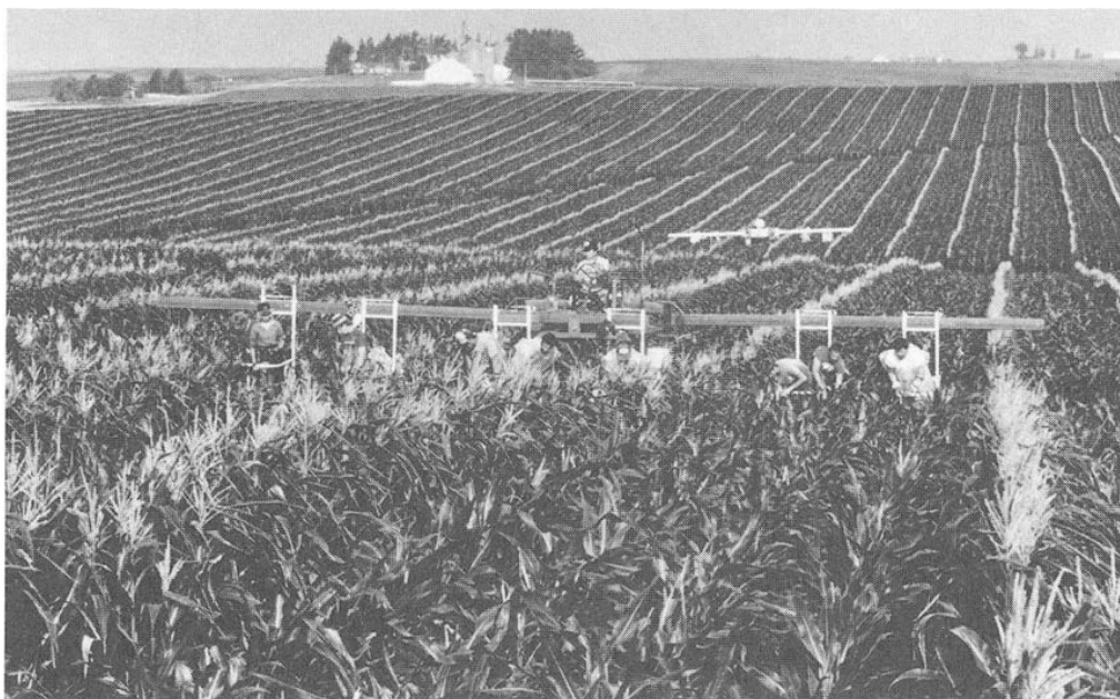
Fig. 9-4. A high clearance personnel carrier transporting detasslers through a seed production field. This view depicts the “second pass” through this field; during this trip, late-emerging tassels are removed.
