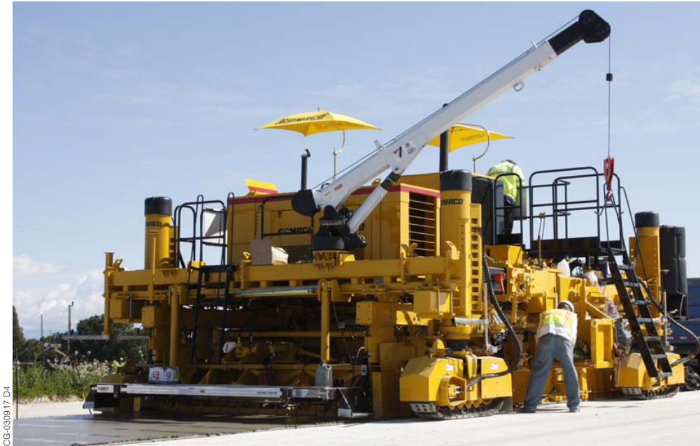
The IDBI attachment is powered by its own C4.4, Tier 3, diesel Caterpillar engine with 91 horsepower (68 kW) @ 2300 rpm.
