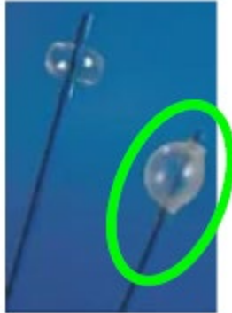
“Figure 6. Offering less precision, an elastomeric balloon (right) will often expand asymmetrically compared with a high-pressure, thin-walled balloon (left).”
