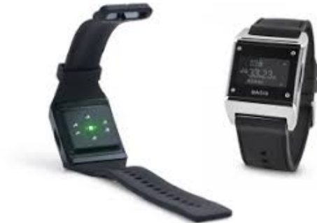
Figure 6 Basis B1 smartwatch from Basis Science was equipped with an optical heart rate sensor 27
