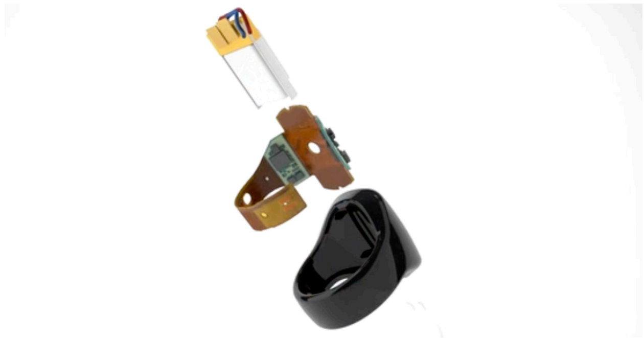
Figure 24 Oura Ring Gen 1 with straight battery 91
