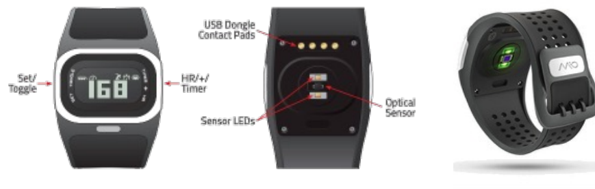
Figure 5 Mio Alpha with the optical sensor lit up 21 22
