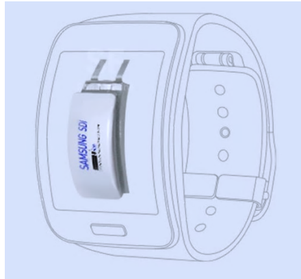
Figure 9 Samsung SDI's curved battery for wearables 47
