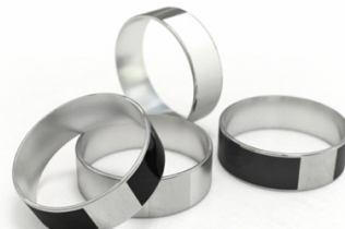
Figure 2 McLear's initial NFC Ring, launched in 2013. Notice the NFC portion, which is signified by the colored (black, grey, or white) portion of the ring 8
