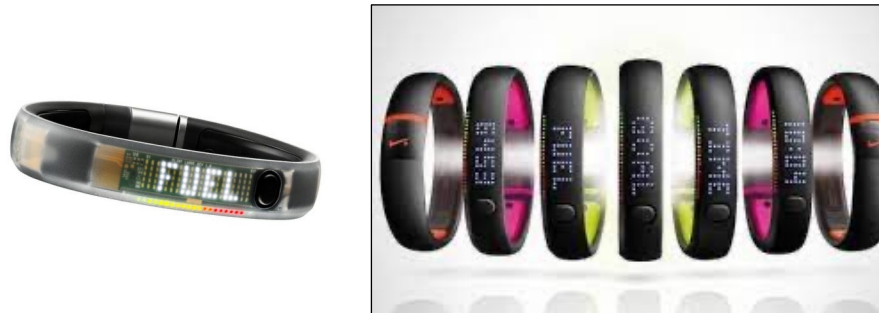
Figure 11 Nike+ Fuel Band Ice (right) reveals the inner workings of the tracker, notably a flexible PCB. Potential messages displayed on the Nike+ Fuel Band (left)
