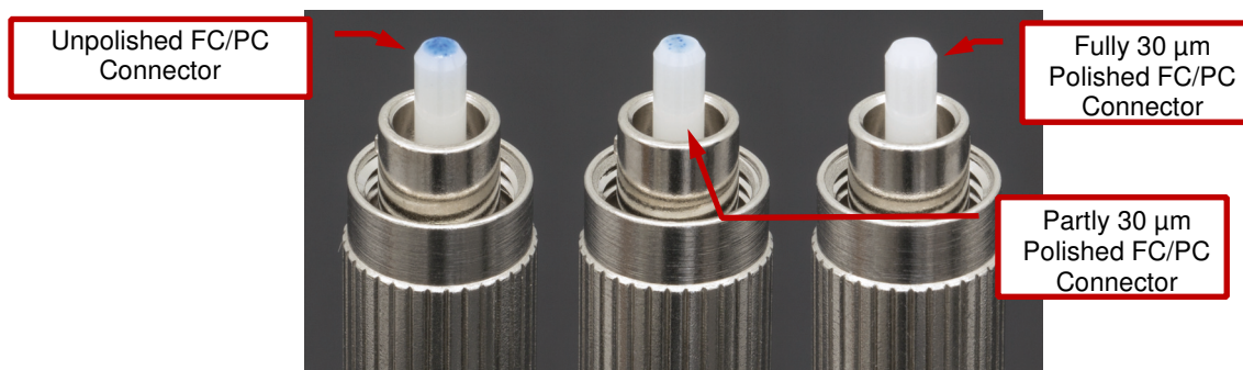
Figure 20 Three FC/PC connectors, from left to right, showing an unpolished, partly polished, and completely polished fiber using the 30 µm polishing film.
