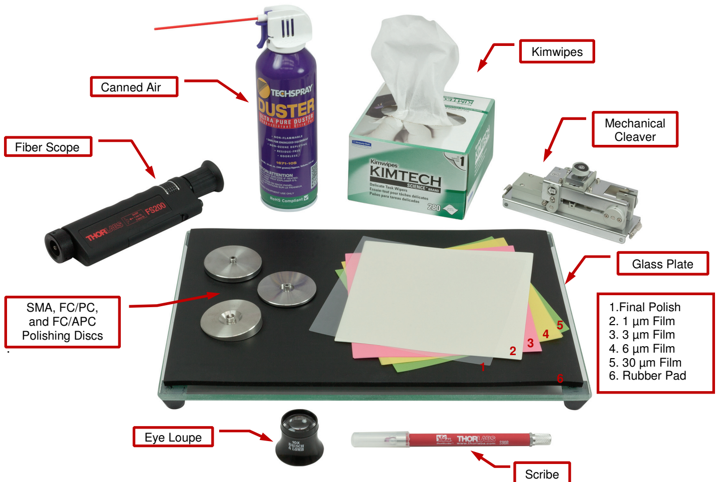
Figure 15 Manual optical fiber polishing parts available from Thorlabs.
