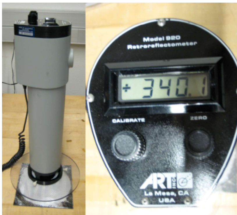
Figure 3-16: Retroreflectometer; Detail of calibration knobs and readout
