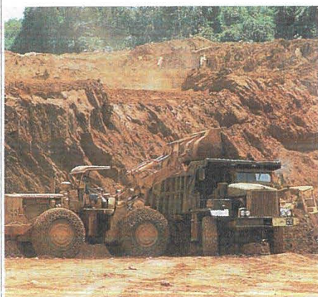
▲ A bauxite mine. Bauxite contains \text{Al}_2\text{O}_3 , the main source of aluminum.
