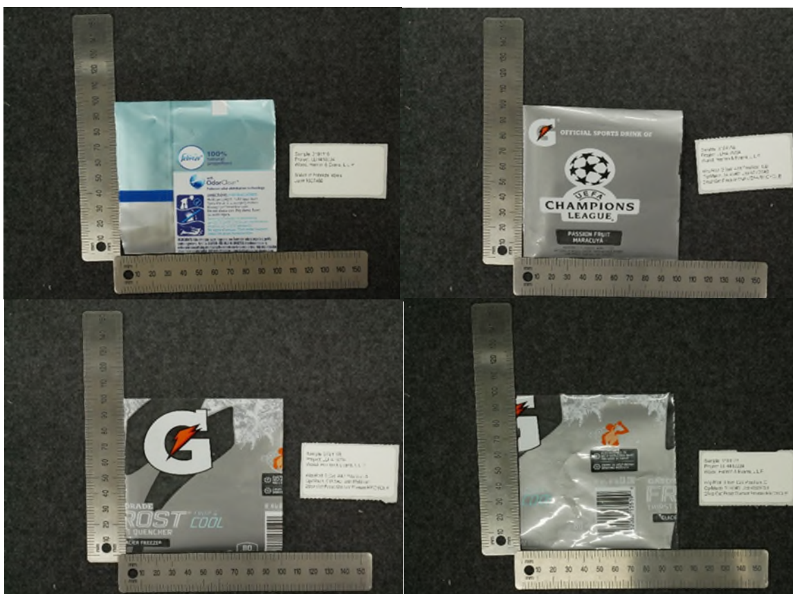
Figure 17. Photographs of cut section of 3191115, 3191158, 3191168, and 3191171 before shrink testing.
