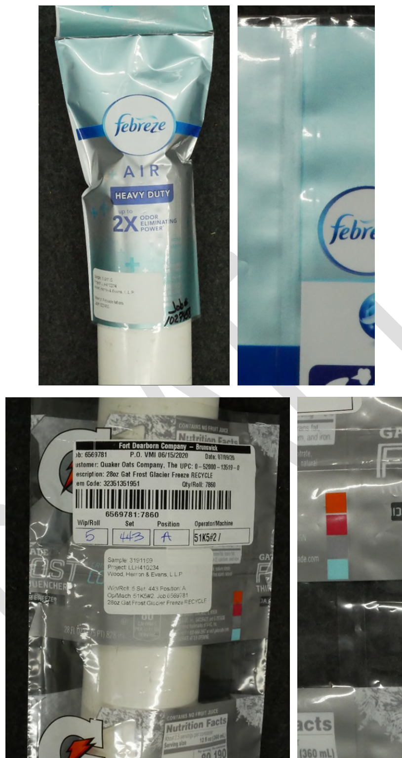
Figure 16. Representative As Received photographs of samples 3191115 and 3191169 representing that all received samples are a tube or sleeve. Close up images show the seam.
