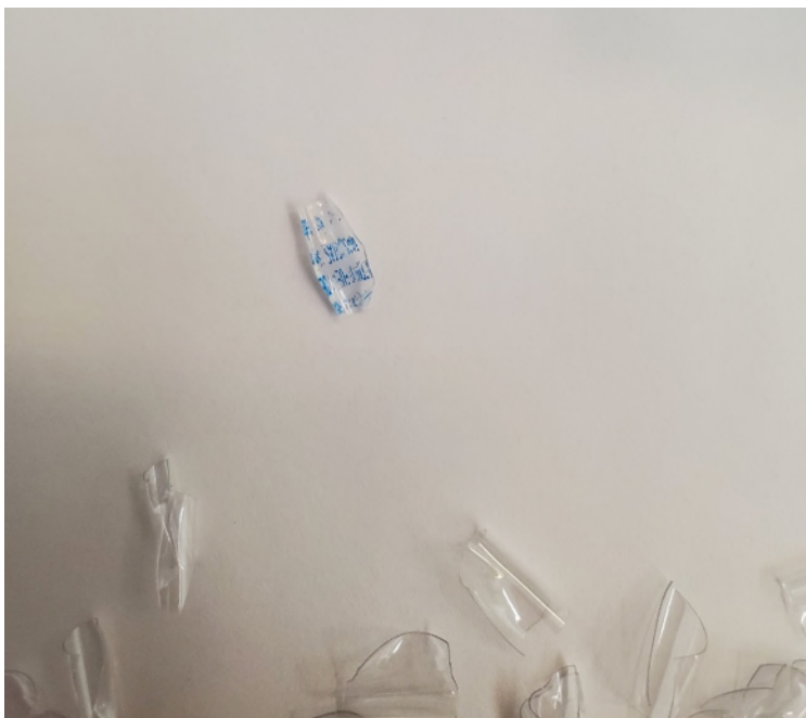
Figure 11a. Representative image 3191115 after caustic wash, warm water wash, float test, and drying.
