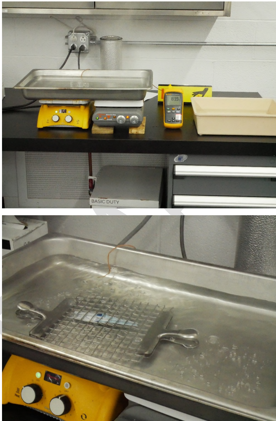
Figure 18. Photographs of experimental setup for shrink testing.
