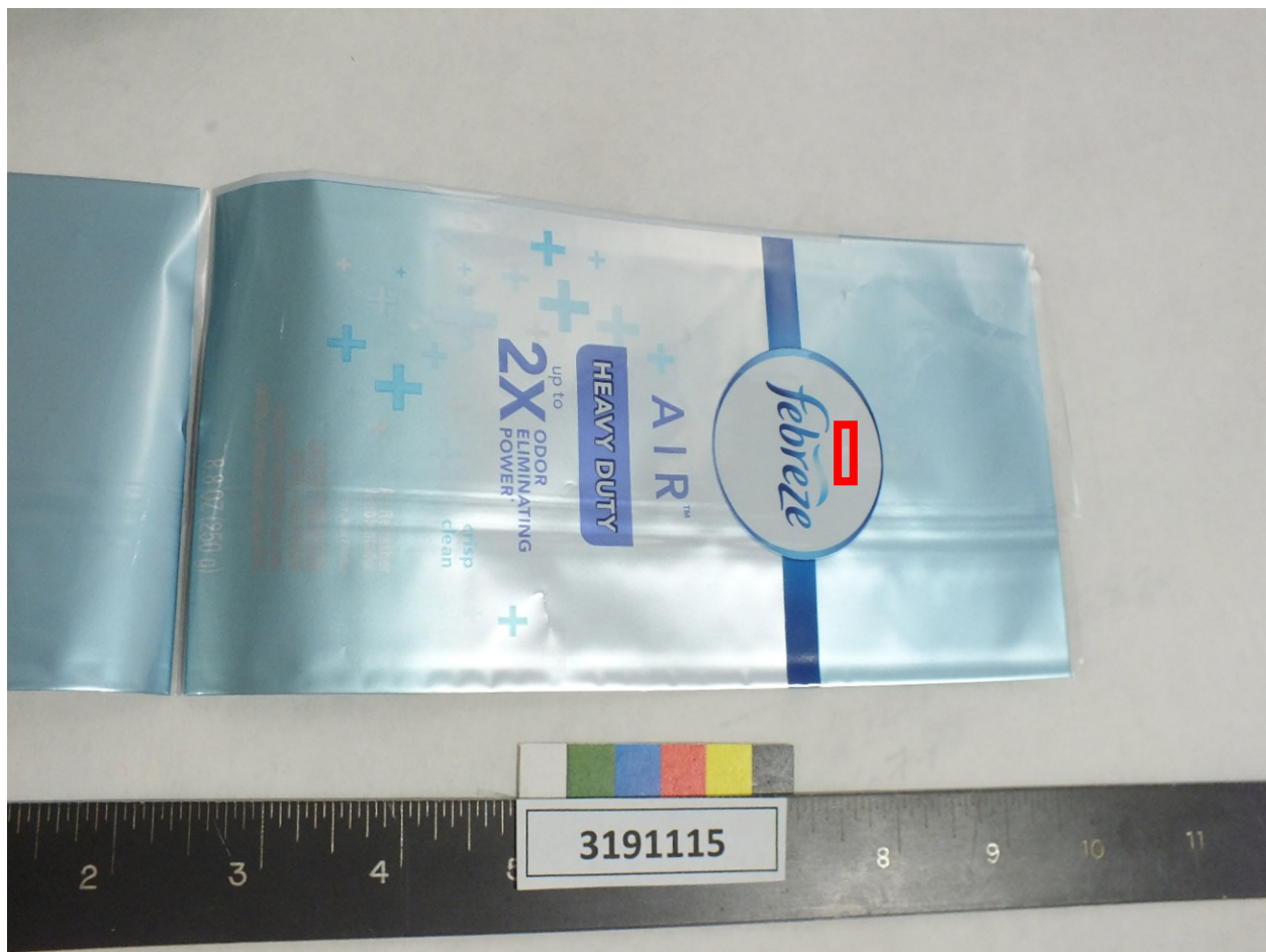
Figure 4. Location of each cross section taken from 3191115, 3191157, 3191167, and 3191176.
