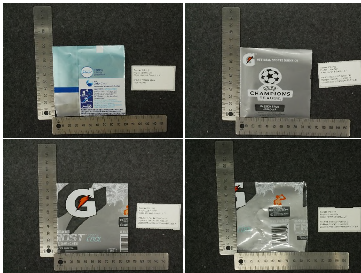
Figure 17. Photographs of cut sections of 3191115, 3191158, 3191168, and 3191171 before shrink testing.
