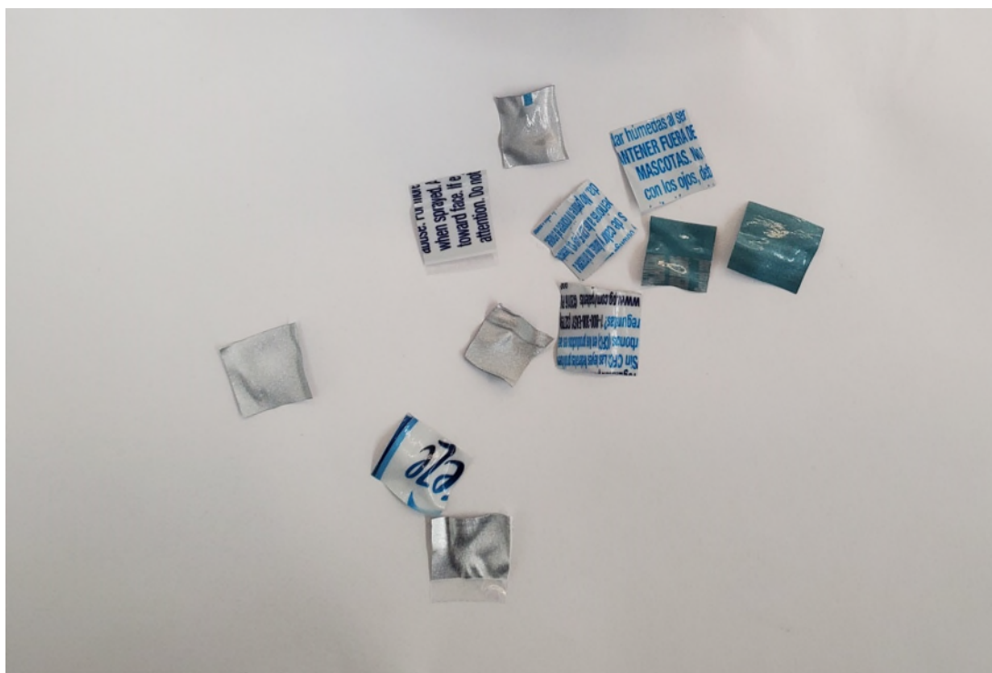
Figure 8 (cont). Representative image of preshrunk 3191115 cut into approximately one square centimeter flakes.
