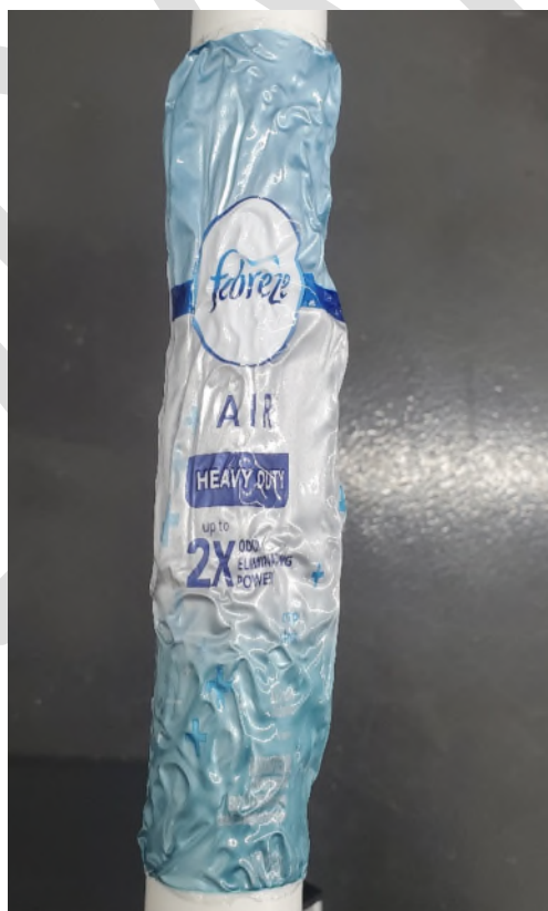
Figure 8. Representative images of 3191115 being shrunk around a 1" pipe.
