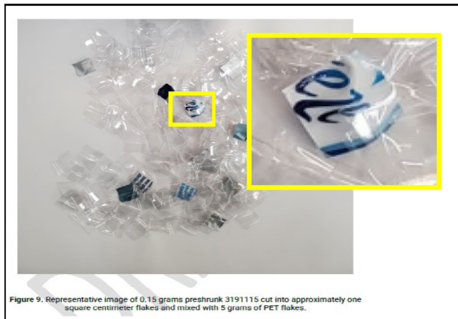
EX1014 Fig. 9 with blowup of label flake used in Petitioner's recyclability testing
