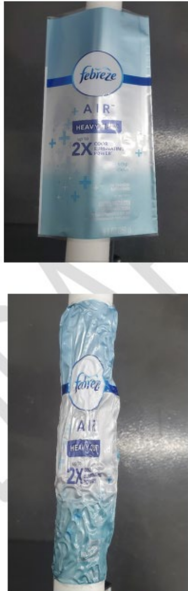
Figure 8. Representative images of 3191115 being shrunk around a 1" pipe.
