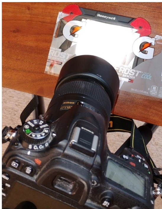
FIG 8: Photographic setup for magnified view of labels. A back light was created by placing a white piece of paper over a Honeywell light, then placing the Gatorade label over the white piece of paper. Photographs were acquired from the top-down perspective, and all digital images were adjusted automatically for clarity and brightness using the “auto color” feature. The images were cropped to show the sections that were best in focus in the image.
