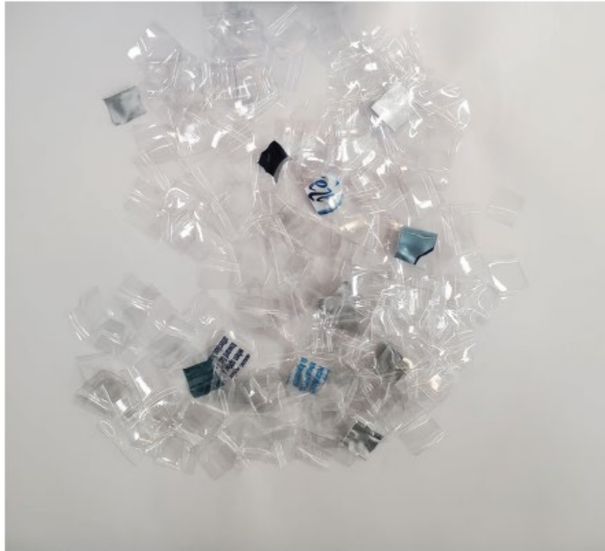
Figure 9. Representative image of 0.15 grams preshrunk 3191115 cut into approximately one square centimeter flakes and mixed with 5 grams of PET flakes.
