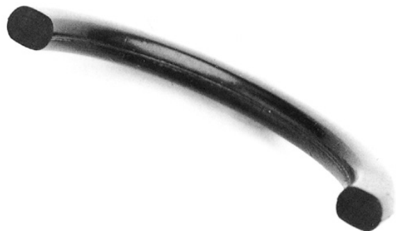
Fig. 10.8 Damage pattern caused by high compression set
