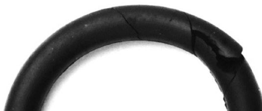
Fig. 10.10 Twisted O-ring with cuts in surface
