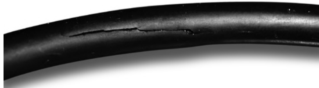
Fig. 10.11 O-ring damaged by explosive decompression
