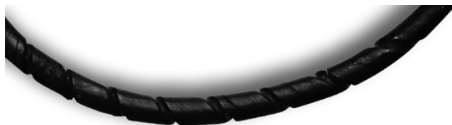
Fig. 10.9 Twisted O-ring with spiral markings
