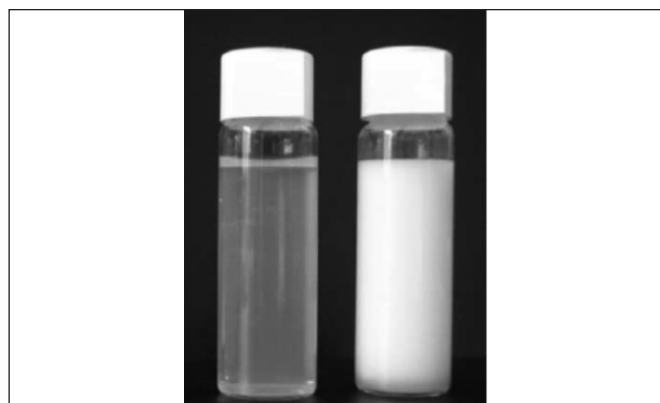
Figure 1 - Optical appearance of a nanoemulsion (on the left, droplet diameters around 35 nm) and a macroemulsion (on the right, droplet size around 1,000 nm). Picture reprinted from reference [20] with permission from Elsevier.
