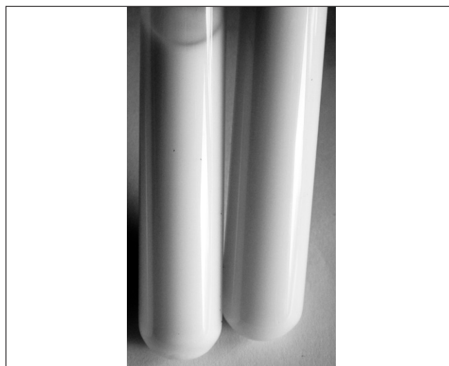
Figure 7 - Picture of a lecithin-based nanoemulsion with particle sizes around 150 nm.
