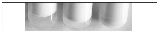
Figure 8 - Destabilisation phenomena in lecithin-based nanoemulsions (yellowish colour, appearance of an aqueous solution). However, redispersion is possible and particle sizes remain stable.
