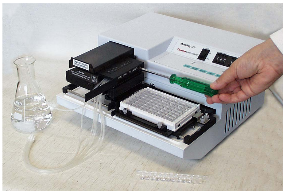
Fig. 7.10 Screwing the calibration screw according to the calibration results
