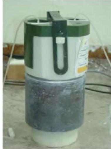
FIG 19. Left: A column generator in its lead shield. Elution is performed by a vacuum vial, also in a lead shield. Right: A typical lead-shielded and closed radionuclide generator.
