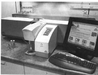
FIGURE 4.3 Mastersizer 2000E particle size analyzer. (Courtesy of Malvern Instruments Ltd.)
