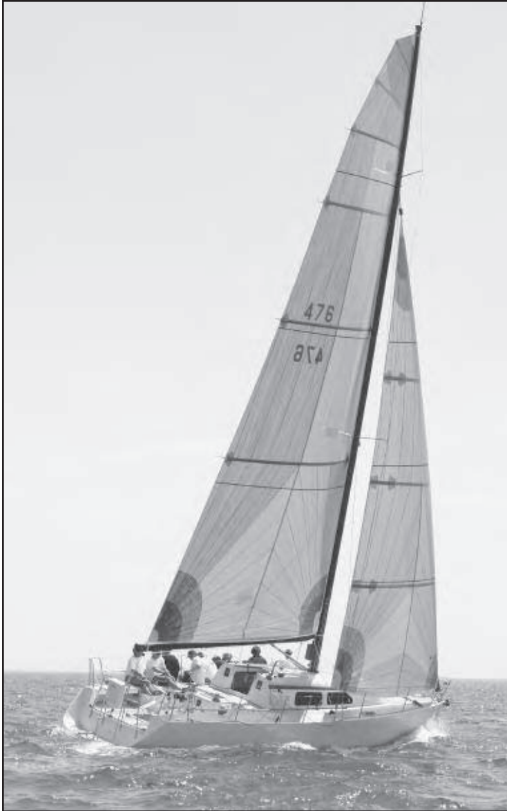
All the telltales on the leech of this mainsail are flying indicating that the sail is trimmed perfectly.
