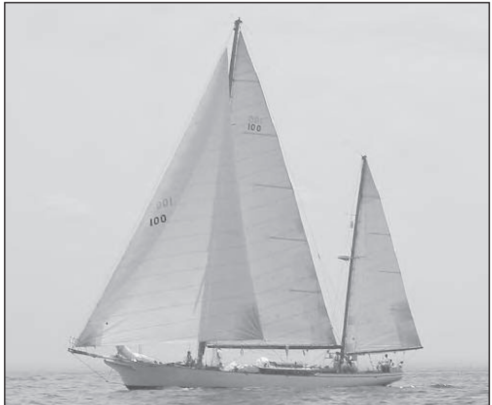
In an effort to improve Dacron, Hood Sailmakers began manufacturing narrow panel fabric seen here in this classic ketch.
