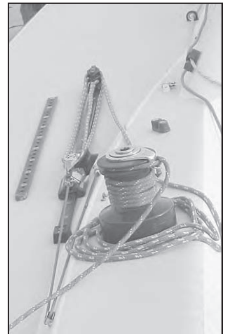
Two systems for adjusting the lead position of a headsail, both using a simple block and tackle for moving the car.
