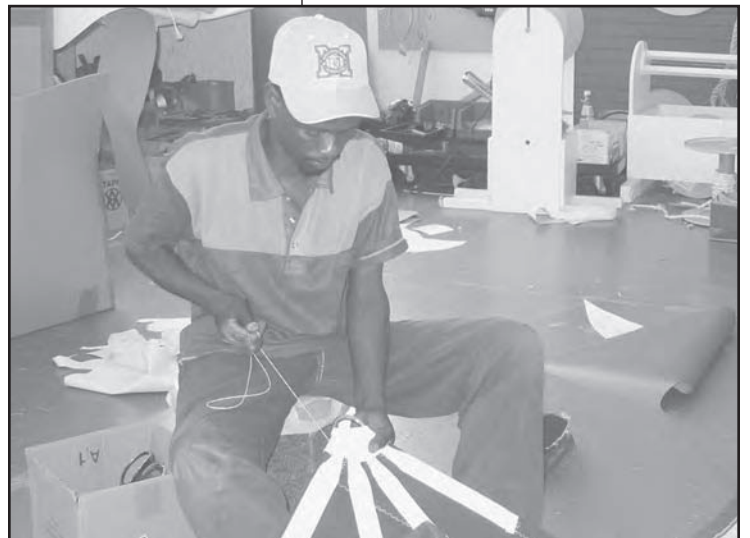
Hand sewing leather on corners is time consuming and tedious, but the wax threads lend an air of tradition to a sail and add durability.
