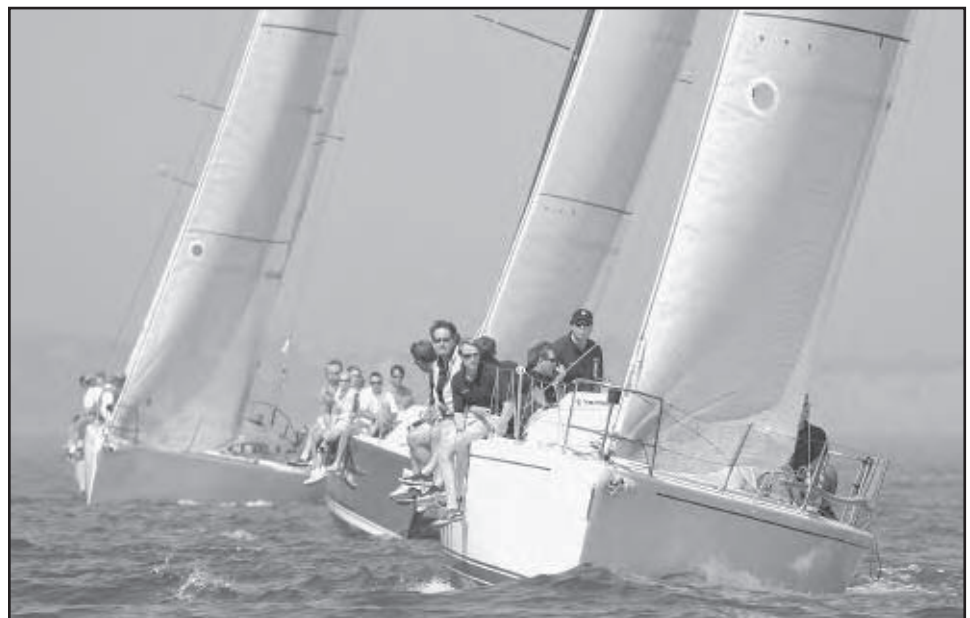
Three good examples of telltales on the luffs of headsails. The windows help.
