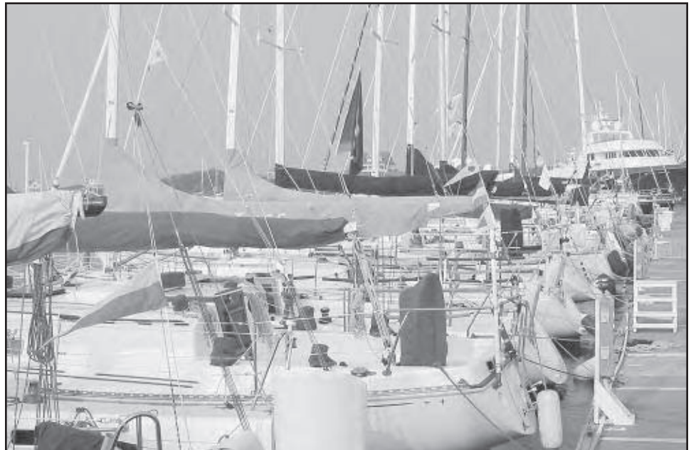
Mainsail covers not only make a boat look neater, but they add life the sail, especially in hot climates where ultraviolet light can damage sails.
