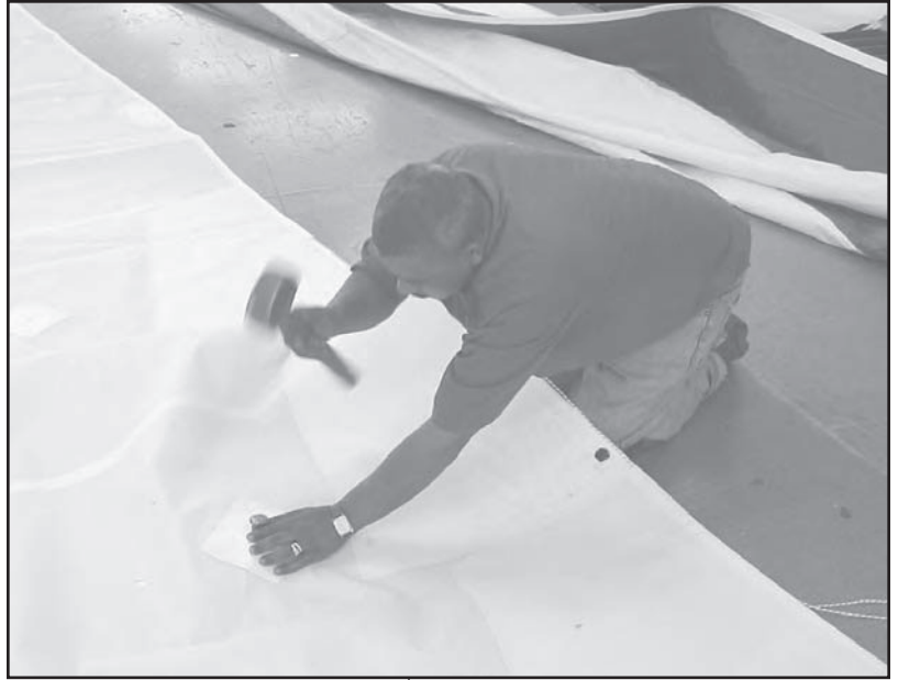
A worker uses a mallet to bang in reef rings in a mainsail.
