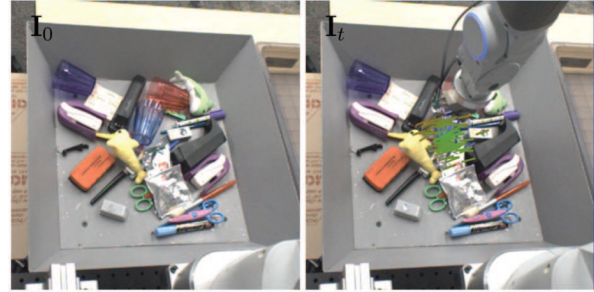
Fig. 3. Example input image pair provided to the network, overlaid with lines to indicate sampled target grasp positions. Colors indicate the probability of success: green is 1.0 and red is 0.0. The grasp positions are projected onto the image using a known calibration only for visualization. The network does not receive the projections of these poses onto the image; only offsets from the current gripper position in the frame of the robot.
