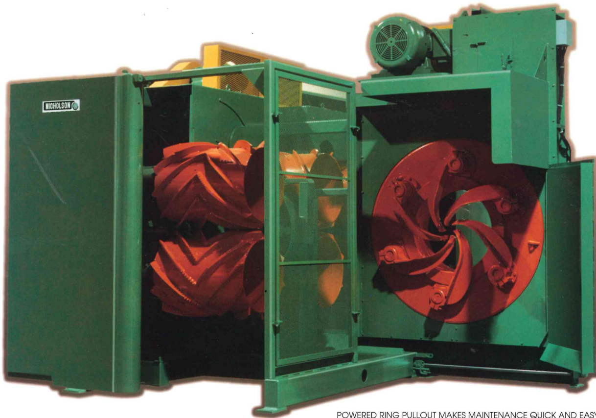
POWERED RING PULLOUT MAKES MAINTENANCE QUICK AND EASY
