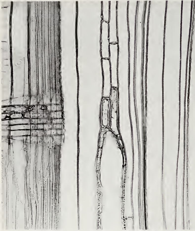
Figure 4-8 Strand tracheids in western larch ( Larix occidentalis Nutt.). The strands become epithelial cells near the resin canal. (120×)
