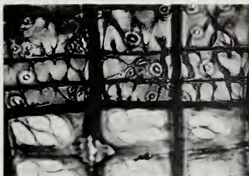
Figure 11-33 Radial section of the wood of longleaf pine, Pinus palustris Mill., showing a portion of a ray composed of three rows of dentate ray tracheids at the top and one complete row of ray parenchyma cells. The latter cells possess cross fields with several pinoid pits having acute apices. (300×)
