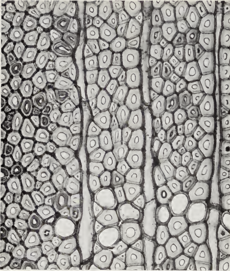
Figure 5-10 Gelatinous (dark-colored) and normal fibers in white oak ( Quercus alba L.). (450×) (Photomicrograph by S. Williams.)
