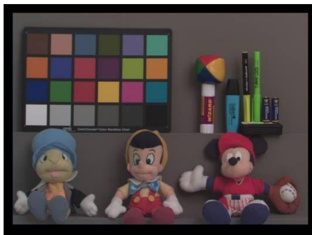
Fig. 8. First color image with metal/dielectric filters patterned in 1.75\mu\text{m} pixels on CMOS, without IR filter.
