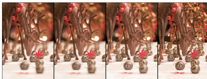
f/3.2, dof = 0.024m f/5.6, dof = 0.043m f/11, dof = 0.086m f/22, dof = 0.172m Focal length 105mm, Focus Distance 1.5m
