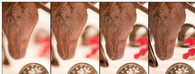
f/3.2, dof = 0.002m f/5.6, dof = 0.004m f/11, dof = 0.007m f/22, dof = 0.014m Focal Length 105mm, Focus Distance 0.47m
