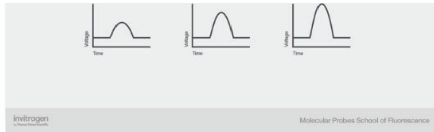
Figure 4. Voltage pulse for forward scatter on three different sizes of cells.
