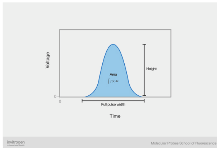
Figure 3. Anatomy of the voltage pulse.
