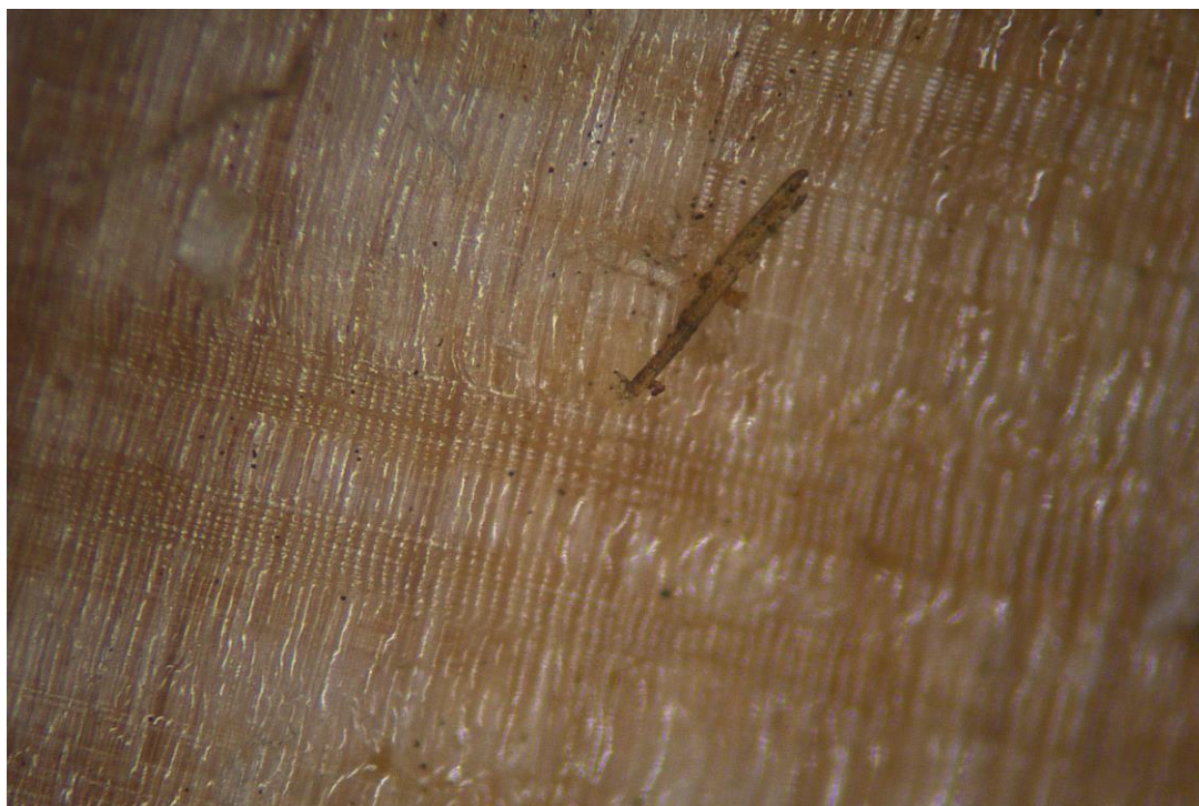
Figure 7-4: DCOI - UP50, Treatment 3. Radial View of cookie with a 40x magnification after it was removed from the pilot plant.
