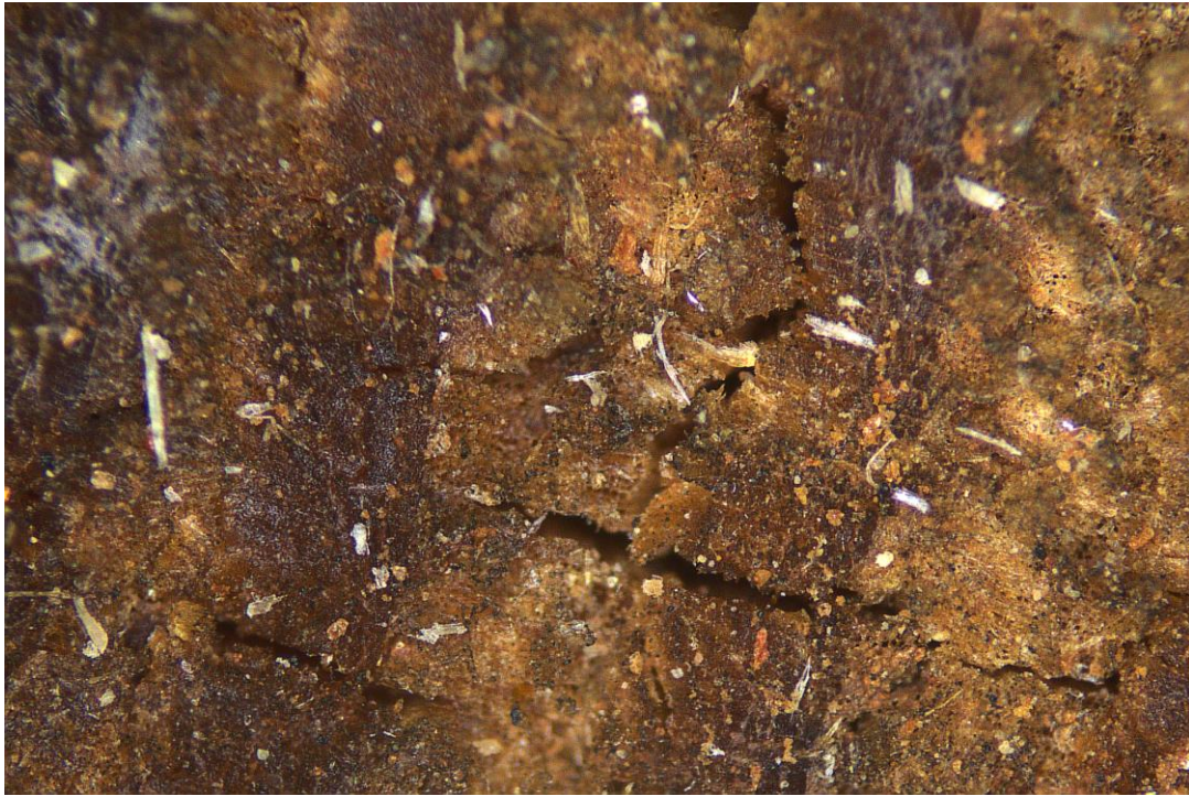
Figure 8-1: DCOI - UP50, Treatment 4. View of cross-section of cookie with a 20x magnification after it was removed from the pilot plant.
