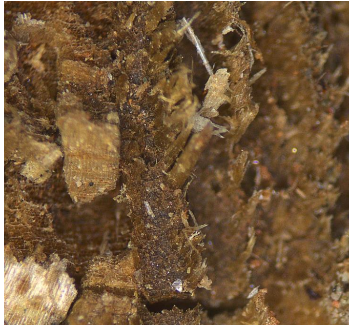
Figure 5-1: DCOI – UP50 , Treatment 1. View of cross-section of cookie with a 20x magnification after it was removed from the pilot plant.
