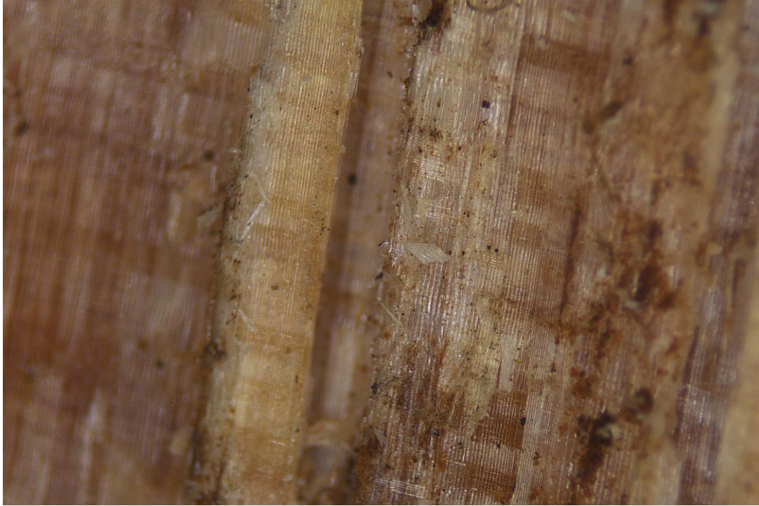
Figure 8-3: DCOI - UP50, Treatment 4. Radial View of cookie with a 20x magnification after it was removed from the pilot plant.
