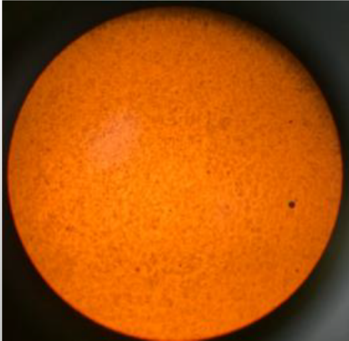
UP - 50 Treatment 5, Initial Solution No gel present in solution
