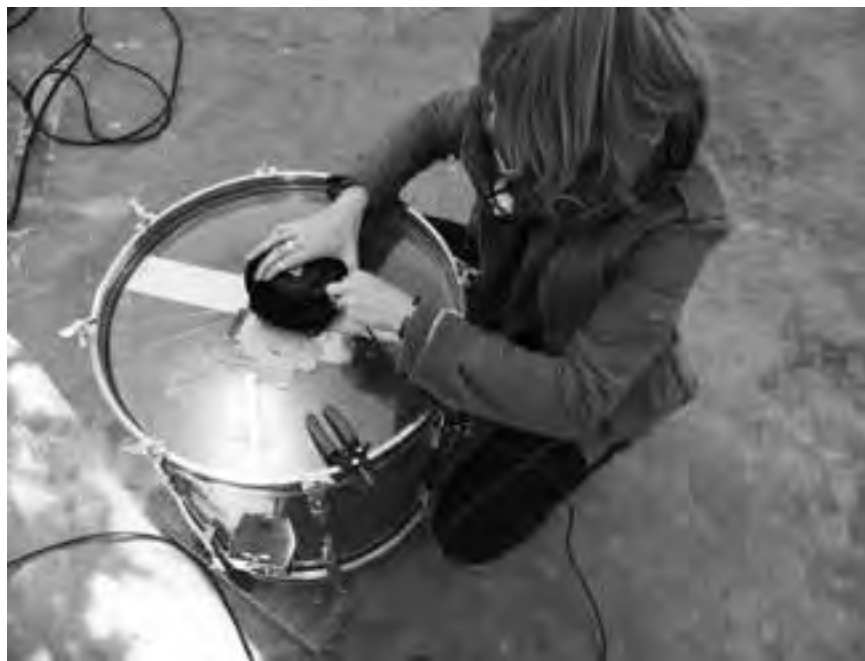
Figure 4.6 Sabrina Schroeder attaches a tactile transducer to a drum. The clear fishing lines are used for keeping the transducer in place during performance. © Sabrina Schroeder. Photo by Phillip Schulze.
