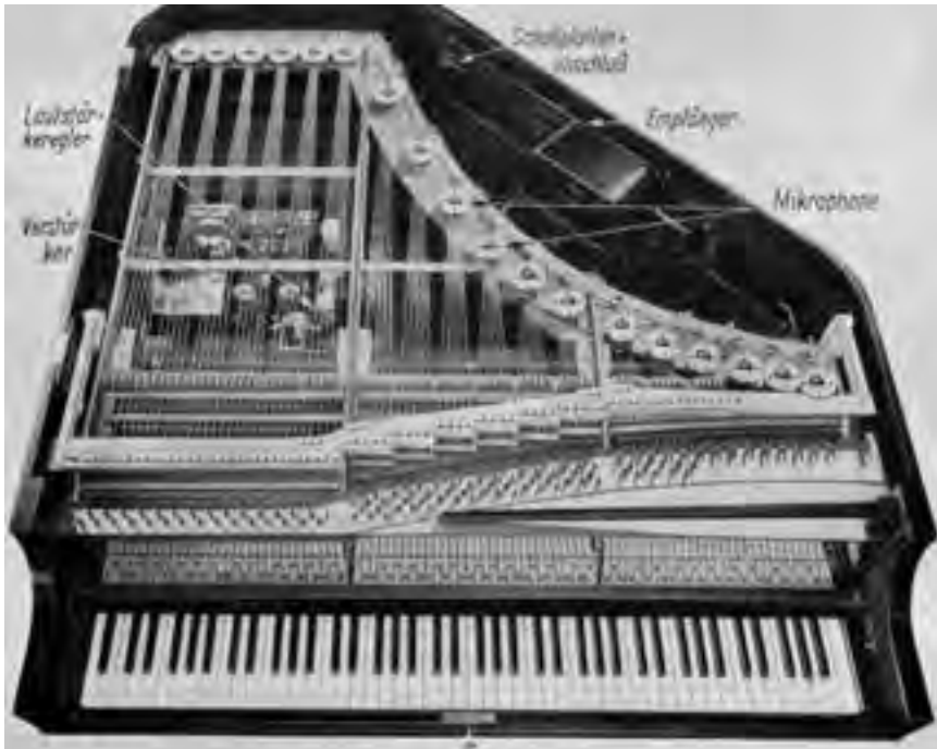
Figure 3.8 The core elements of the Neo Bechstein: an amplifier ( Verstärker ), a volume slider ( Lautstärkereger ), a connection for a gramophone ( Schallplattenanschluß ), a radio ( Empfänger ) and electro-magnets ( Mikrophon ) (Winckel 1931, 840).
