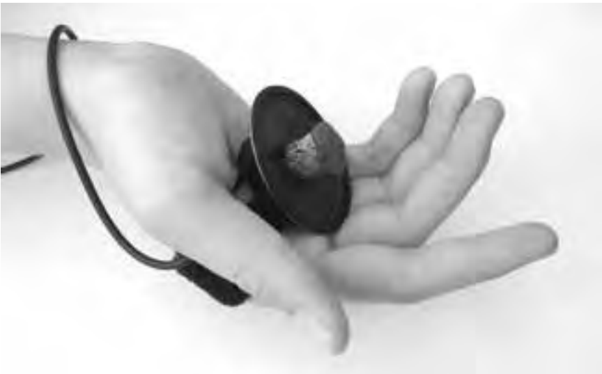
Figure 5.2 A cork with felt on top is attached to the dust cap of this small loudspeaker used by Ute Wassermann to facilitate contact with the gong. © Ute Wassermann. Photo by Ute Wassermann.
