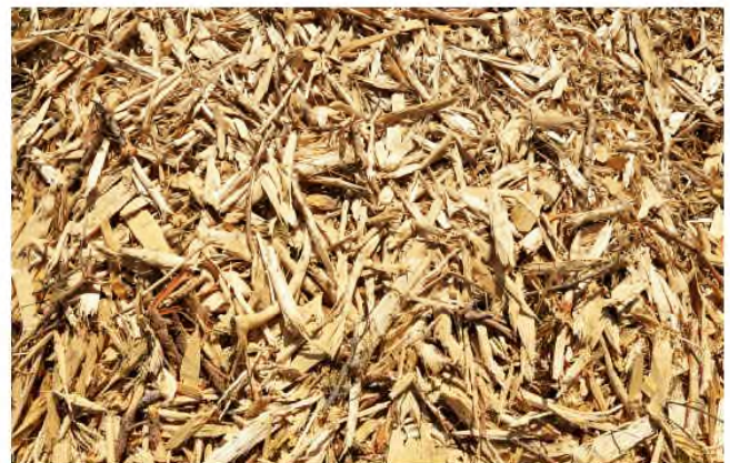
Logs are converted into wood chips before undergoing the kraft pulping process.
